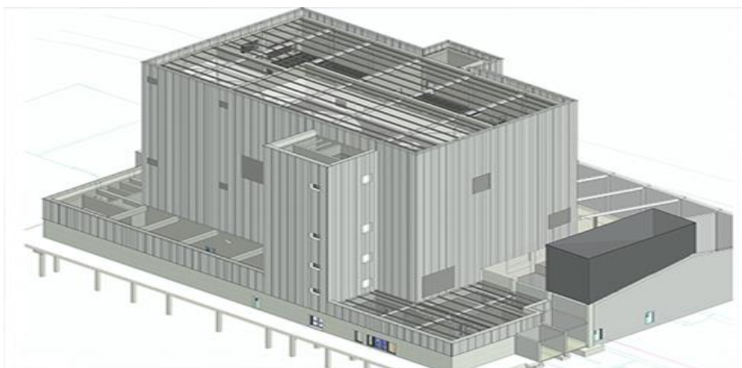
Fig. 7 Perspective view of the digital construction model of the new Tipperary evaporator plant (source https://www.johnpaul.ie current 08/05/2020 ©John Paul Construction)
